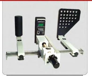
The LigMaster<sup>™</sup> is an instrumented arthromer that can provide a fast and easy assessment of ligament function for joints of the shoulder, knee, ankle and elbow.
