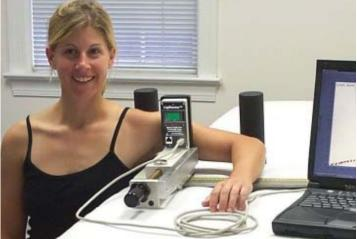
The LigMaster<sup>™</sup> software, which runs on a PC computer or laptop, collects force response joint motion data from the electronic sensors and displays the data as a graph of force vs. strain, force vs. displacement or force vs. inversion/eversion (ankle joint only).
